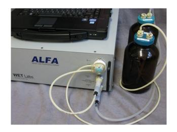
Use aluminum foil to cover the bottles and hold the tubing in position.
