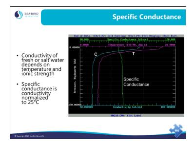
The conductivity of fresh or salt water is strongly dependent on temperature, as shown above by the similarity in the shape of the C and T plots. Specific conductance is typically used for fresh water applications, where the salinity equation is out-of-range. It allows us to visualize the conductivity without the temperature dependence, providing some indication of the amount of salts in the water.
