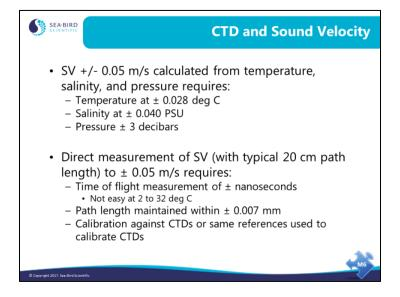
Sound velocity (SV) sensors measure the flight time of a pulse of sound between transducers. To meet the  $\pm\,0.05$  m/s specification of a typical 20 cm path SV sensor, the time of flight must be measured to within about 4 nanoseconds. The electronics to perform this are difficult but feasible; however, the time delays associated with the acoustic transducers cannot be maintained over pressure and temperature.
