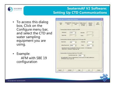
The CTD communications form allows you to select the communications parameters for your instrument as well as data transfer protocol and header options. Instruments with older firmware revisions are not able to change baud rate during data transfers.
