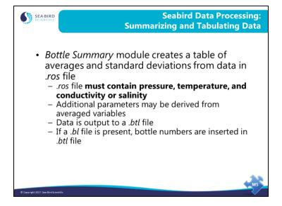
The .ros file created by Data Conversion contains a set of data scans for each water sample taken. The Bottle Summary module takes the process one step further by averaging the scans for each water sample into a single line of data that contains averages and standard deviations for each of the parameters in the .ros file. In addition, you may add derived parameters to this list. The derived parameters are calculated from the averages of the data contained in the .ros file.
