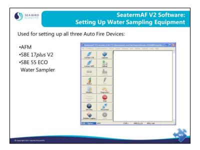
SeatermAF V2 includes a simple interface for entering bottle closure parameters, and transfers that information to the auto-fire equipment. It is also used to set up the SBE 19, 19*plus*, 19*plus* V2, 25, 25*plus*, or 50 for operation, and to upload data from the auto-fire equipment (AFM, SBE 17*plus* V2, or SBE 55 ECO Water Sampler) and CTD.
