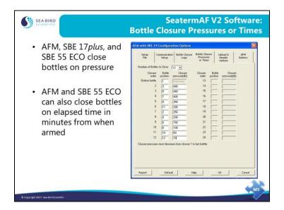
Once you have defined the governing bottle closure logic – on upcast, on downcast, when stationary, or on elapsed time – you need to enter the number of bottles to close and which bottle to close when. Bottles may be closed in any order desired.
