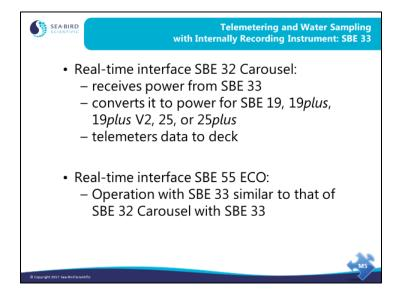
The SBE 33 provides power and telemetry for internally recording instruments. Telemetry capability is over 10 km of sea cable.
