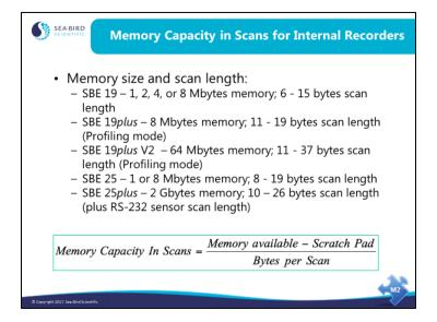
Because our profiling instruments can be set up to acquire data from auxiliary sensors, the *length* of data for each sample is dependent on the number of auxiliary sensors that are *enabled* (the CTD manual provides the commands for *enabling* the auxiliary sensor channels). The number of samples that fit in memory is dependent on the length of data for each sample, as well as the memory size in the CTD.
