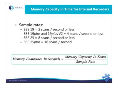
Memory endurance in time is the ratio of memory capacity in scans divided by the instrument sample rate.
