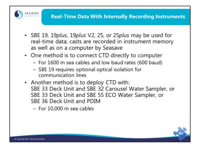
SBE 19s may be outfitted with high power cable drivers and optical isolation for transmitting real-time data. The SBE 19plus, 19plus V2, 25, and 25plus come standard with this equipment. With the addition of a Deck Unit and associated underwater equipment listed above, the data telemetry is the same as discussed for the SBE 911plus.
