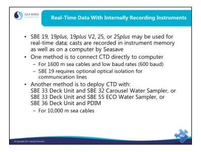
Unlike the SBE 19 and 25, the SBE 19 plus, 19 plus V2, and 25 plus **do not** have to be asleep when you move the magnetic switch to the On position.
