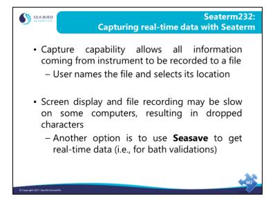
The capture capability allows Seaterm232 to place all characters received into a file. This is useful for testing instruments, performing diagnostics, or in some cases recording real-time data. Note that there is no testing of data integrity and the act of displaying the characters on the screen while they are being written to a file may cause some characters to be lost.
