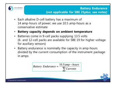
Battery endurance is difficult to estimate, because a battery's life depends on the ambient temperature. Moreover, batteries tend to lose their capacity as they age. The information on this slide is a good rule of thumb for alkaline batteries. However, for critical work, consider that batteries are cheap, so you might as well start with a new set.
