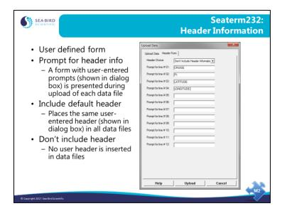
Now we are looking at the Header Form tab from the dialog box shown in the previous slide. User headers may be placed in uploaded data files, to provide more details about the conditions of the cast.
