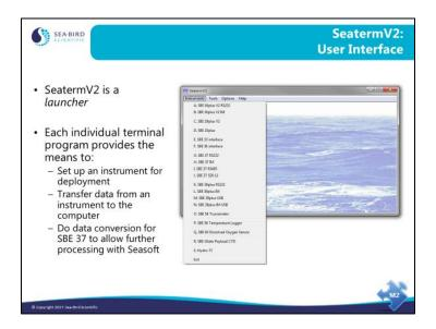
SeatermV2 is a terminal program *launcher* for use with instruments developed or redesigned in 2006 and later. The common feature of this generation of instruments is the ability to output data in XML. SeatermV2 launches one of the following terminal programs, depending on the communication protocol required:
