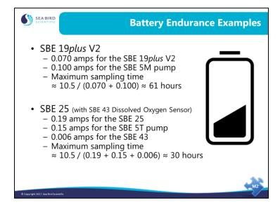
Where do you find the information on current draws? See the specifications in the CTD manual for the CTD and pump; see Sea-Bird brochures / specification sheets for any auxiliary sensors (such as the SBE 43, etc.). For any *third party* sensors (such as a WET Labs fluorometer, Teledyne Benthos altimeter, etc.), see the brochure / specification sheet provided by the manufacturer. You must include all of the current draws for all of the sensors being powered by the CTD.
