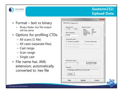
When you click the Upload menu in Seaterm232, you start a process that produces an upload file that is compatible with our data processing software (SBE Data Processing).
