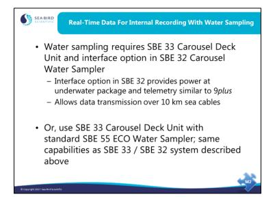
The SBE 19, 19plus, 19plus V2, 25, and 25plus can be equipped with water sampling equipment. The SBE 33 Carousel Deck Unit and SBE 32 Carousel (or SBE 55 ECO) provides power and telemetry for the CTD very similar to the 11plus / 9plus setup. In addition to water sampling, this equipment allows data telemetry over 10 km of sea cable and supplies more than enough power for the CTD and auxiliary sensors.
