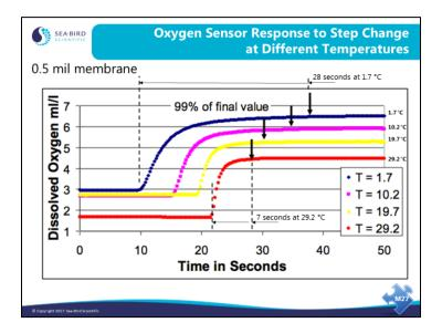
The plot above illustrates the effect that temperature has on a dissolved oxygen sensor. The colder the water that the sensor is working in, the longer it requires to come to a final value. In profiling applications this phenomenon is observable as upcast and downcast hysteresis.
