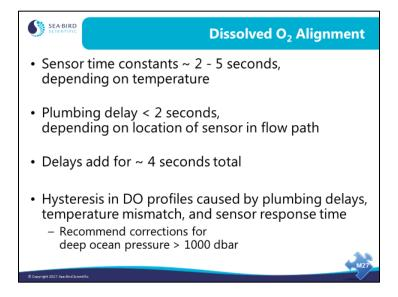
Aligning oxygen current and temperature in relation to pressure can improve hysteresis (mismatch) in dissolved oxygen profiles. The SBE 43 has a faster time constant and shows improvement in hysteresis over the Beckman- or YSI-type of sensor. Deep-ocean hysteresis corrections are advised at depths greater than 1000 dbar
