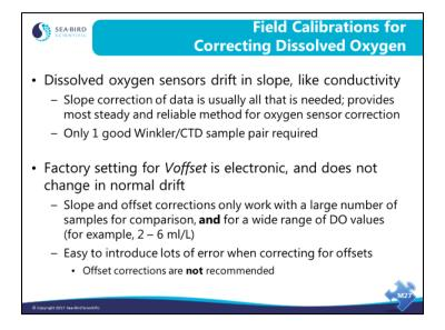
Terms that can be modified by the user to adjust the calibration of the SBE 43:
