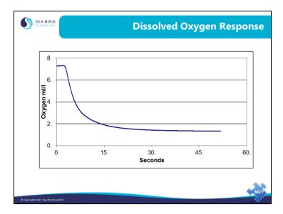
This graph (and the graphs on the following pages) is for an SBE 43 with a 0.5 mil membrane. The 0.5 mil membrane is recommended for profiling applications. Sea-Bird also offers a 1 mil membrane for moored applications
