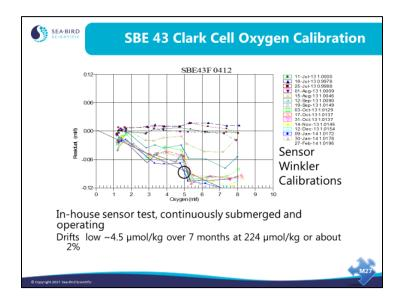
Plot indicates a slope drift of < 0.1 ml/L (~4.5 umol/kg) over seven months at saturation
