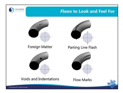
Any of these flaws may result in the instrument flooding.
