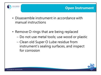
Make sure the instrument is completely dry before opening. Water on the electronic circuits can severely damage the instrument.
