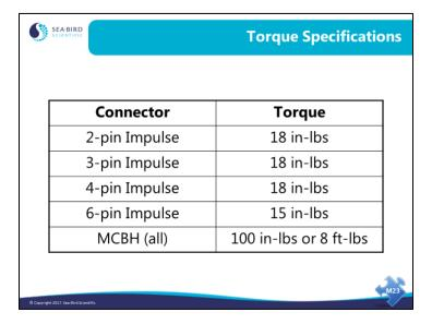
Impulse connectors are our *standard* connectors. MCBH connectors are wet-pluggable connectors, and are optional on all of our instruments.
