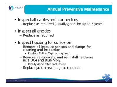
Inspect cables for cuts, abrasions, cracking, and corrosion. Sea-Bird recommends that you replace *worn* cables, even if they are still functional (save working cables as spares).
