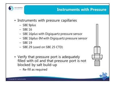
Sea-Bird can provide a pressure sensor oil refill kit, PN 50025, for these instruments. *Application Note 12-1: Pressure Port Oil Refill Procedure & Nylon Capillary Fitting Replacement* provides the details on use of the kit.
