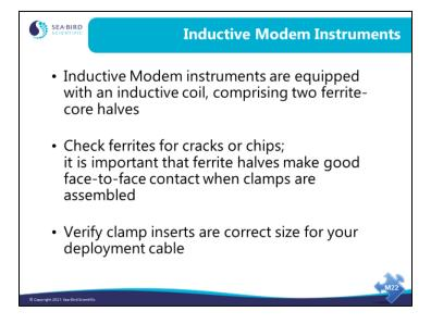
Proper communications with an IM instrument requires that the ferrites are not damaged, and that the two modem halves mate closely (< 0.1 mm gap). Note that if the clamp inserts are too small for the cable, there will be a gap between the modem halves. An attempt to reduce the gap may damage the cable or modem if the bolts are over-tightened.
