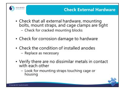
Excess corrosion on anodes can negate their effectiveness.
