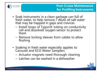
Post-cruise maintenance is very important to the longevity of the instrument. Trapped salt water will form crystals as it dries; these crystals can eventually cause damage to both housings and O-rings.
