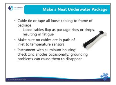
Neatness counts! Secure all your loose cables. When you lower your instrument package at 1 meter per second, any loose cabling will flap. This sort of repetitive motion will fatigue the cables and shorten their working life.
