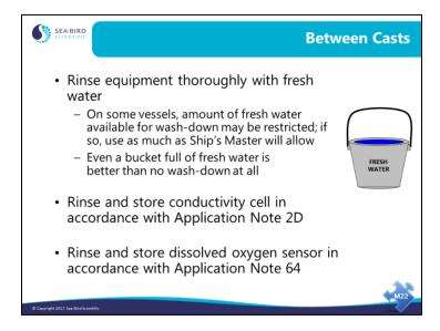
Most ships have both freshwater and saltwater wash-down hose connections. Make sure you are using the freshwater.
