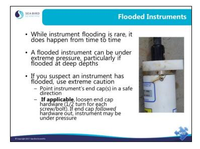
Loosening the end cap hardware to test if the instrument is under pressure is only applicable to instruments that attach to the housing through the **top** of the end cap (for example, SBE 9*plus*, 25, 17*plus*, 26, 26*plus*, 53, 54).
