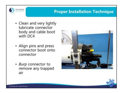
Align the dimple on the connector boot with the large pin on the connector. Remember to *burp* the connector(s) after installation.
