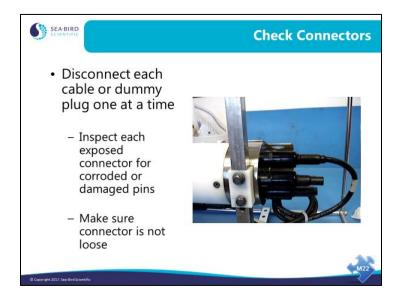
Application Note 57: Connector Care and Cable Installation on our website is a good resource for connector cleaning and installation, and also provides cold weather installation tips.
