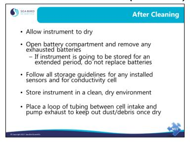
If batteries leak in the battery compartment, battery bulkhead replacement needs to be performed at Sea-Bird.
