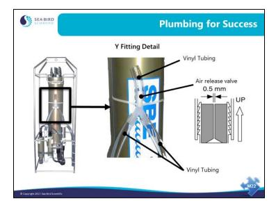
This slide shows the proper way to run the tubing for an instrument in a cage meant to be deployed vertically. Note the highest point in the plumbing is the top of the *Y*; there is a fitting with a small hole in the top of the *Y* that allows the air in the tubing to vent as the instrument goes into the water.
