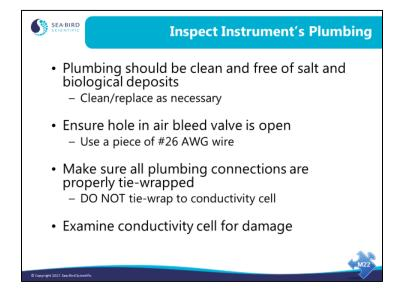
Contaminated plumbing may degrade the initial data.
