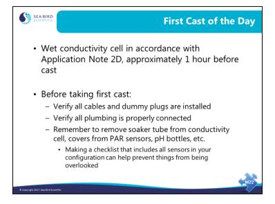
Use a 0.1% Triton X-100 solution to rewet the conductivity cell.
