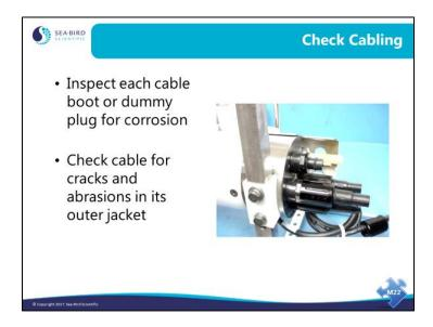
Cables can be damaged by chaffing, extreme bends, or contact with the ship deck or hull (pinching).
