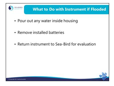
Any details that you can provide to Sea-Bird regarding a flooded instrument are appreciated, especially deployment depth or the depth that good data was lost (modular or real time sensors).
