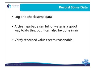
As mentioned on the last slide for the status commands, saving this data will help to verify the instrument was functioning properly before the deployment if troubleshooting is required later.
