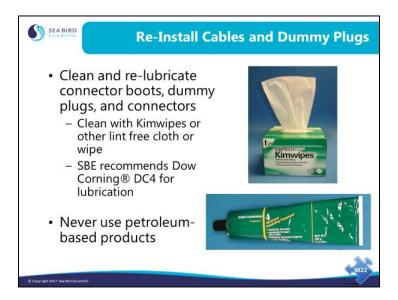
**Do not use WD-40 or other petroleum-based lubricants**; petroleum-based lubricants will damage connectors.
