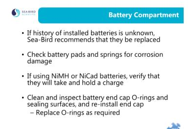
Batteries may have a *good* voltage reading when not under load.
