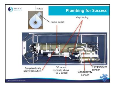
Instruments meant for horizontal deployment are easier to plumb. The pump is oriented so that the outlet is the highest point on the plumbing. Care must be taken to ensure there are no loops in the plumbing that would trap air. Because this system is meant to be deployed horizontally, there is no *sloshing* effect and no requirement for the SBE 9*plus* that the inlet and outlet be at the same height.
