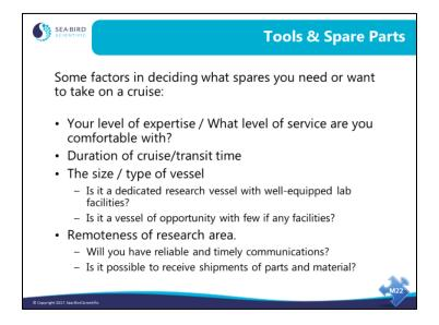
Some spares are not practical as their use requires recalibration of the instrument (for example, spare conductivity cells and spare temperature probes).
