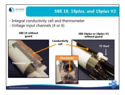
The SBE 19 has side-by-side temperature and conductivity sensors. The SBE 19 plus and 19 plus V2 feature inline sensors and an integral ducting system, which ensures that water that passes the thermometer goes into the conductivity cell.
