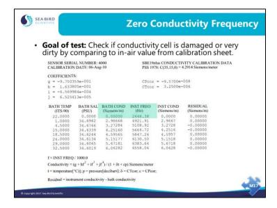
The Zero Conductivity Frequency is provided on the conductivity calibration form we send you with your CTD.
