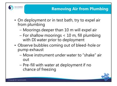
If you do not see air bubbles coming out of the bleed hole, the hole maybe clogged. Use a fine gauge wire to clear the bleed hole.
