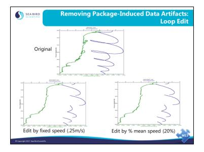
Here is the example of loopy data that we showed earlier. The bottom two plots have been edited by the two means available. Both plots show very similar results. The bottom left plot is made by editing out data that drop below a fixed speed, in this case 0.25m/s. The bottom right plot is made by editing data that drops below 20% of the mean speed calculated over a 5-minute (300-second) window; this method gives you a bit more flexibility.
