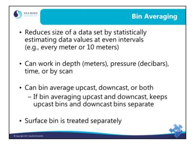
Bin averaging is a means of reducing your data set to a more tractable, and perhaps a more meaningful, size. The Bin Average module makes a statistical estimate of data values at a user-prescribed interval based on the surrounding data. You can bin data on the even meter or 10 meters. You can bin data with a bin size that represents the resolution of your instrument. For time series measurements, you can bin on time interval.
