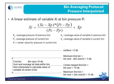
An estimate of each variable is made using the average value of that variable and pressure in the previous bin, and the average values of the variable and pressure in the current bin. Bin averaging with interpolation provides output data at regular intervals (for example, 10 meters, 20 meters, etc.).
