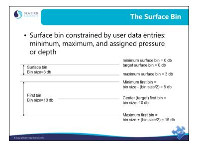
The surface bin is handled differently because the previous bin would be up in the air. The surface bin is assigned a beginning pressure or depth, an ending pressure or depth, and a target pressure or depth.
