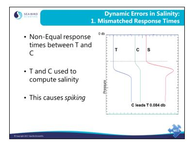
In this example, the conductivity sensor responds to a change faster than the temperature sensor. This causes the salinity to *spike* high of correct.
