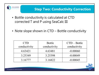
The numbers in the column labeled CTD –  $Bottle\ conductivity$  are not constant. Rather, they have the slope we have been harping on.
