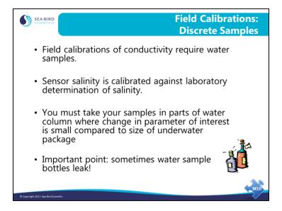
Most instrument packages are more than a meter tall. If you take your samples for field calibrations in a part of the water column where the salinity or oxygen concentration is changing rapidly, you will not get a good sample for calibrating. Not only is there mixing of the water inside the water sampler, but you will be comparing a large mixed sample with a virtual point sample from the sensors.
