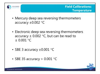
Traditional mercury deep-sea reversing thermometers are not capable of resolving temperature accurately enough to field calibrate the SBE 3. Nor do electronic deep-sea reversing thermometers have the accuracy for field calibrations. Sea-Bird markets a deep-sea standards thermometer, the SBE 35, which has the physical configuration to allow calibration in a triple point cell or a gallium melt cell.
