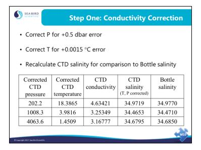
Temperature and pressure are corrected first. CTD salinity is recalculated only for comparison to the bottle salinity. We will be correcting conductivity, not salinity.
