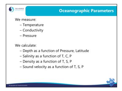
We measure physical quantities with Sea-Bird instruments. These quantities are then used to calculate the many parameters that are found in the analysis of oceanographic data. Because the calculated parameters rely on accurate measurement of the physical quantities, a small error in the original measurement can result in a large error in data analysis.
